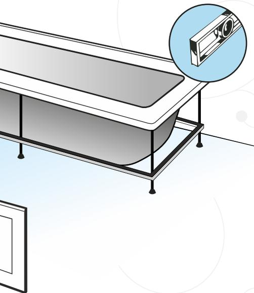
Step a) Set the bathtub in its final position, level it and connect the drainage and overflow valve (optionally, for more stability of the bathtub, you can screw up the plastic feet to the floor)
