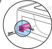
sockets, screwing it up at the corners right and left. (Picture 4)
